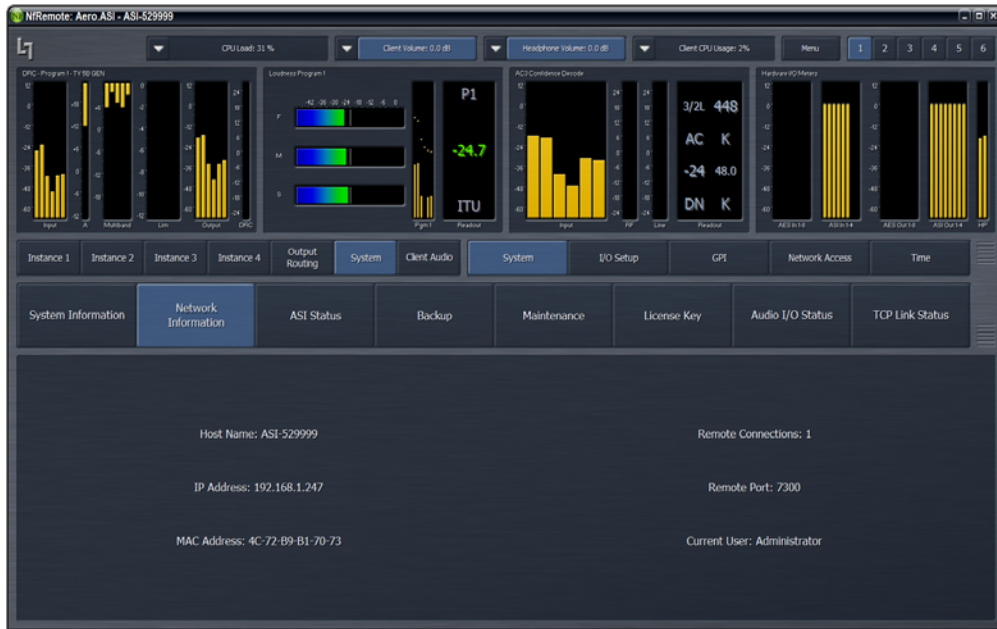
Figure 1-12 IP address, remote port, MAC address, and other system information
