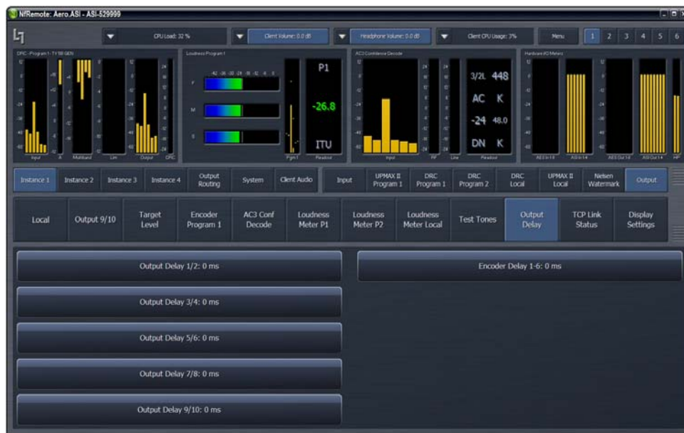
Figure 1-15 Output Delay settings available for each instance
