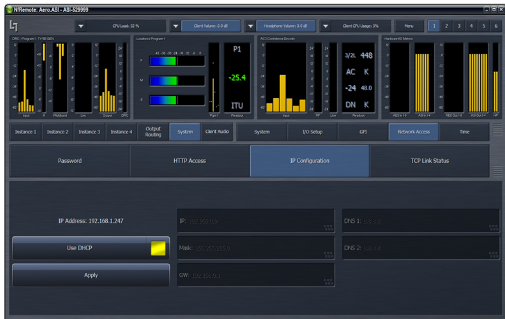
Figure 1-13 Configuring the IP address
