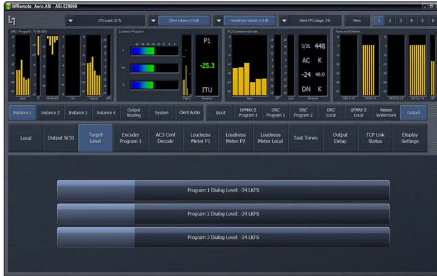
Figure 1-22 Dialog level (dialnorm) is set under the Target Level tab
