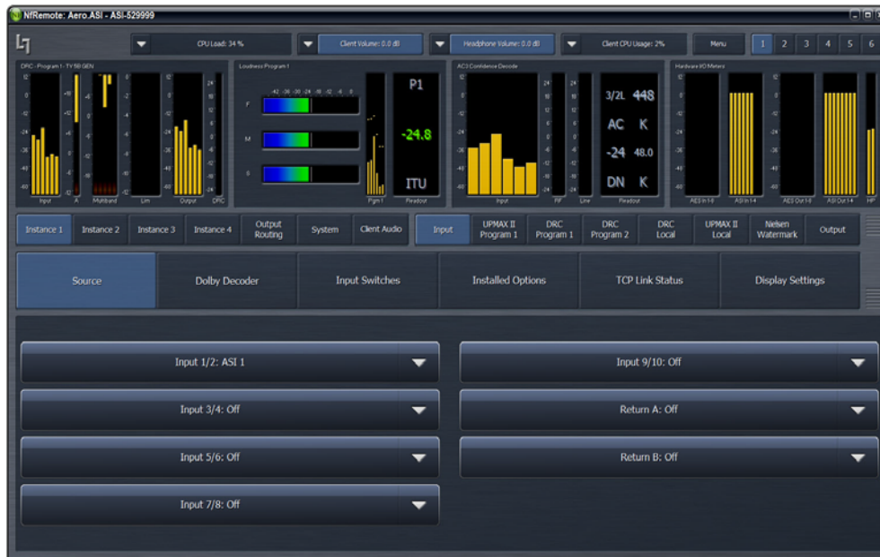
Figure 1-8 Available inputs for 5.1+2+Local instance: 1–6 + 7–8 + 9–10
