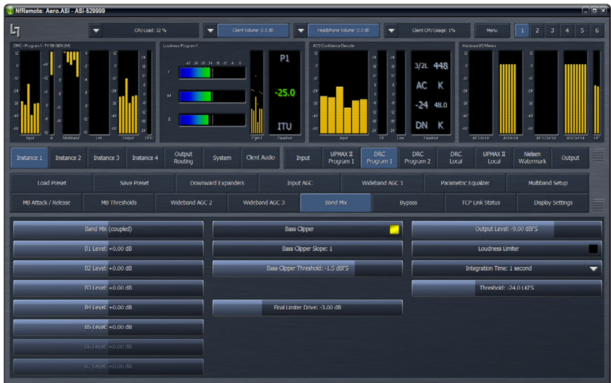
Figure 1-24 Adjusting Output Level so the meter matches the target
