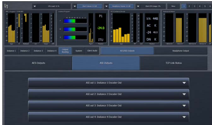
Figure 1-10 The AES and ASI Outputs tabs allow source selection for each physical output
