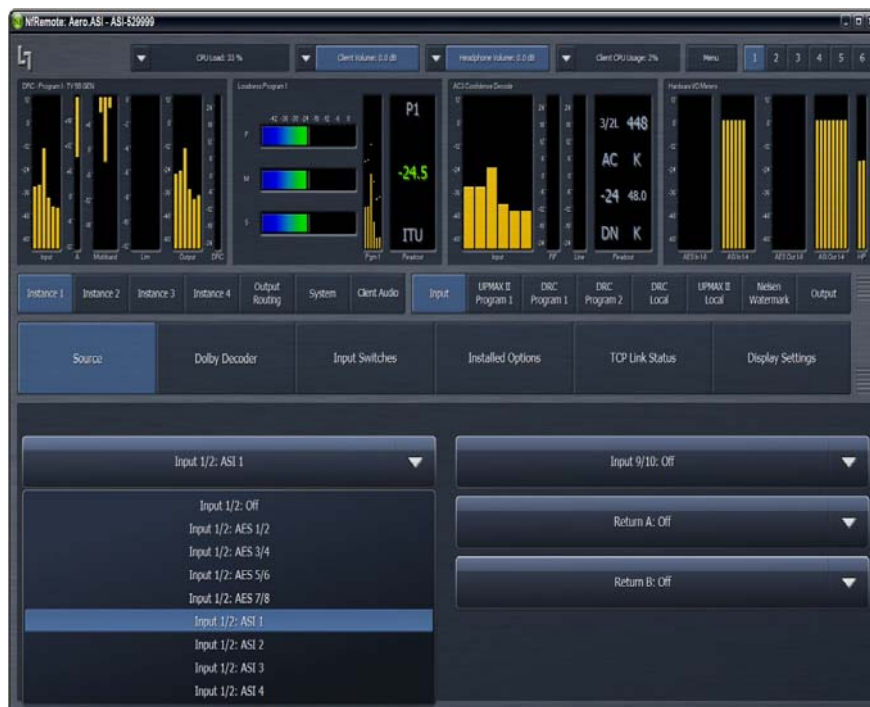
Figure 1-9 Drop-down menu for each Instance input lists all physical inputs
