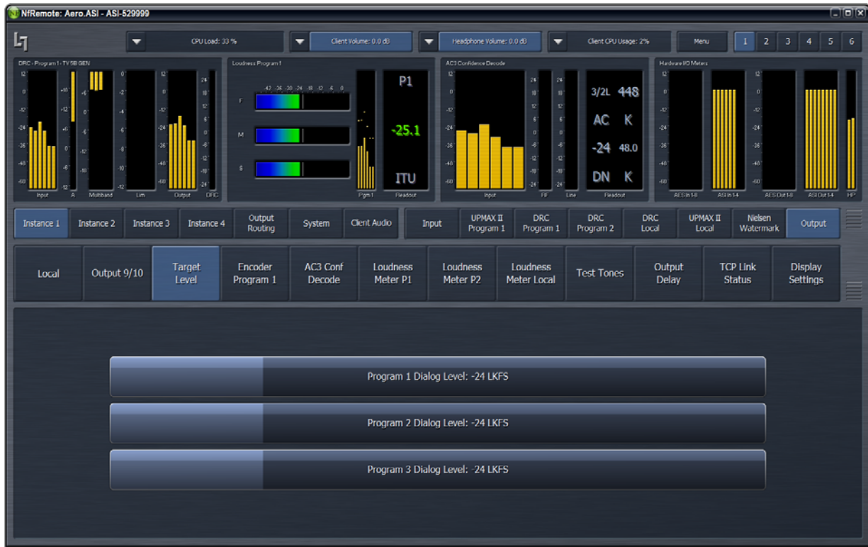
Figure 1-25 Adjusting the target level (dialnorm) to match the meter
